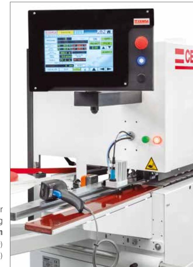
The Optional **double edge feeding**, **barcode reader** and **pneumatic cylinder on infeed fence** can be installed under request in any PRO Series for a greater versatility and an error-free adjustment of the working units.
